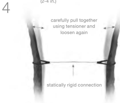
cobra ultrastatic was specifically developed for use for cracked branches. Its very low cable expansion of 0.2% per tonne makes this system ideal for immobilising branches in such situations. It is installed as follows:
