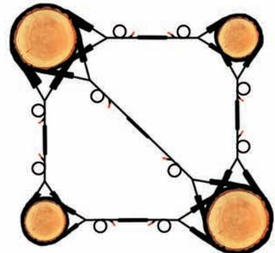
The ring bracing system is usually sufficient.
