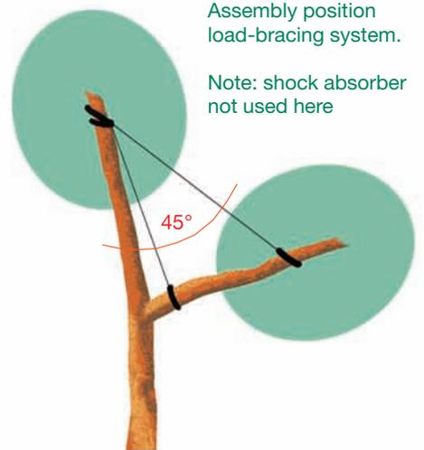
Assembly position load-bracing system.
